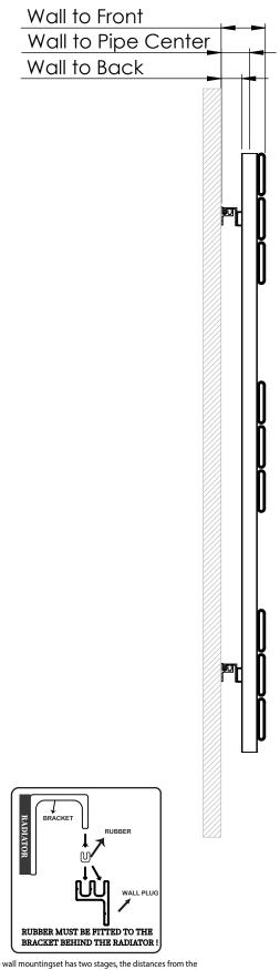
Since the wall mountingset has two stages, the distances from the wall are indicated in the table below according to the two stages
