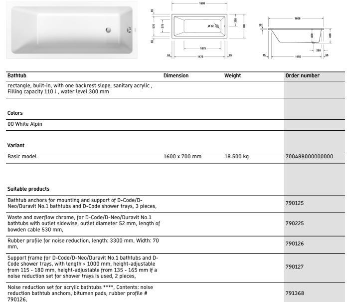
Waste and overflow Quadroval with water inlet, chrome, \*, for<br/>bathtubs with outlet on the side, outlet diameter 52 mm, length<br/>of bowden cable 530 mm,
