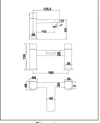
Dimensions (measurements in mm)
