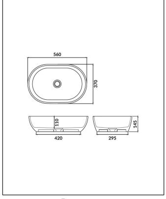
Dimensions (measurements in mm)
